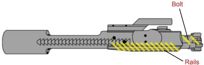
Apply CLP to the front rails on both sides of the bolt carrier and to the bolt where is it highlighted yellow.
