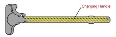
Apply CLP to the top and sides of the charging handle arm where it is highlighted yellow.
