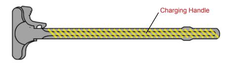
Apply CLP to the top and sides of the charging handle arm where it is highlighted yellow.
